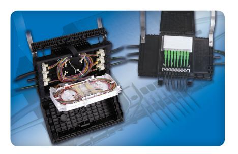
The FDC-B8 is a gel sealed in-line distribution and drop closure designed for FTTx networks. It accommodates up to 2 PLC splitters, 48 fusion splices and 8 SC adapters and has 6 main cable ports and 8 drop cable ports.
