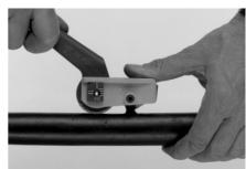
For longitudinal cutting of uncut cable, position the tool and press down the handle. The knife slides through the cable sheath, supported by the footed segment.
