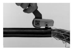
This allows easy slitting from thin to large cables starting from the edge.
