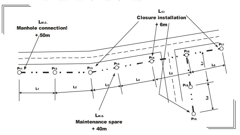
L<sub>M.c.</sub> = excess cable length for manhole connection  $L_{M.s.}$  = excess length created for service purposes
